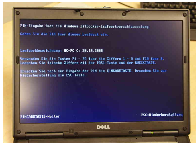
Fig. 1. Spoofed BitLocker PIN-entry screen.
